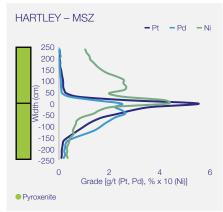
The zone strikes in a north-north-easterly trend and dips between 5° to 20° on the margins flattening towards the axis of the basin. Peak base metal and PGM values are offset vertically with palladium peaking at the base, platinum in the centre and nickel towards the top. Visual identification of the MSZ is difficult.
