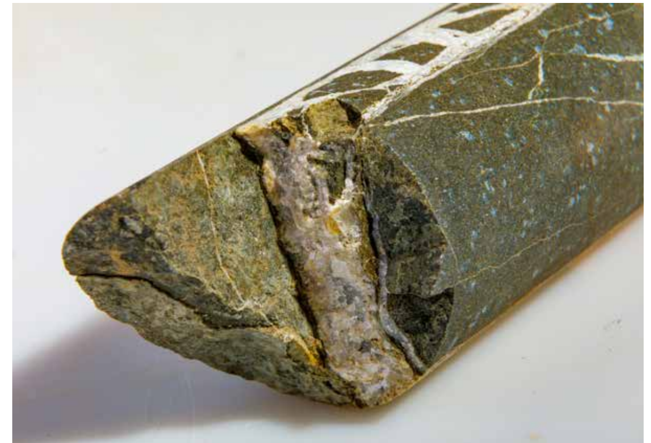
Faulted lamprophyre dyke with calcite vein, exploration core
