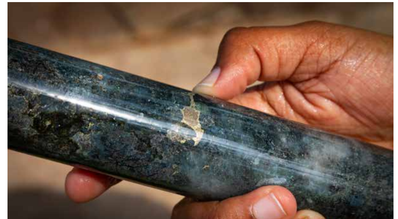
Sulphide mineralisation within exploration core, Merensky reef
