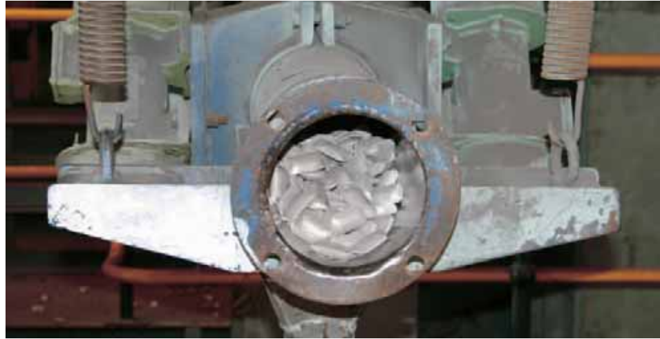
Nickel briquettes in the mouth of the chute, prior to being loaded in drums, at the Base Metals Refinery, Springs.
