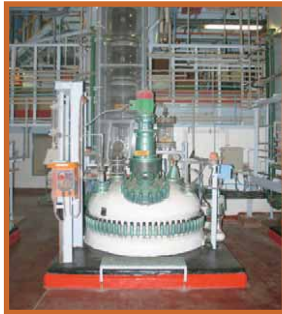
The glass-lined vessels in the platinum production section of the Precious Metals Refinery, Springs.
