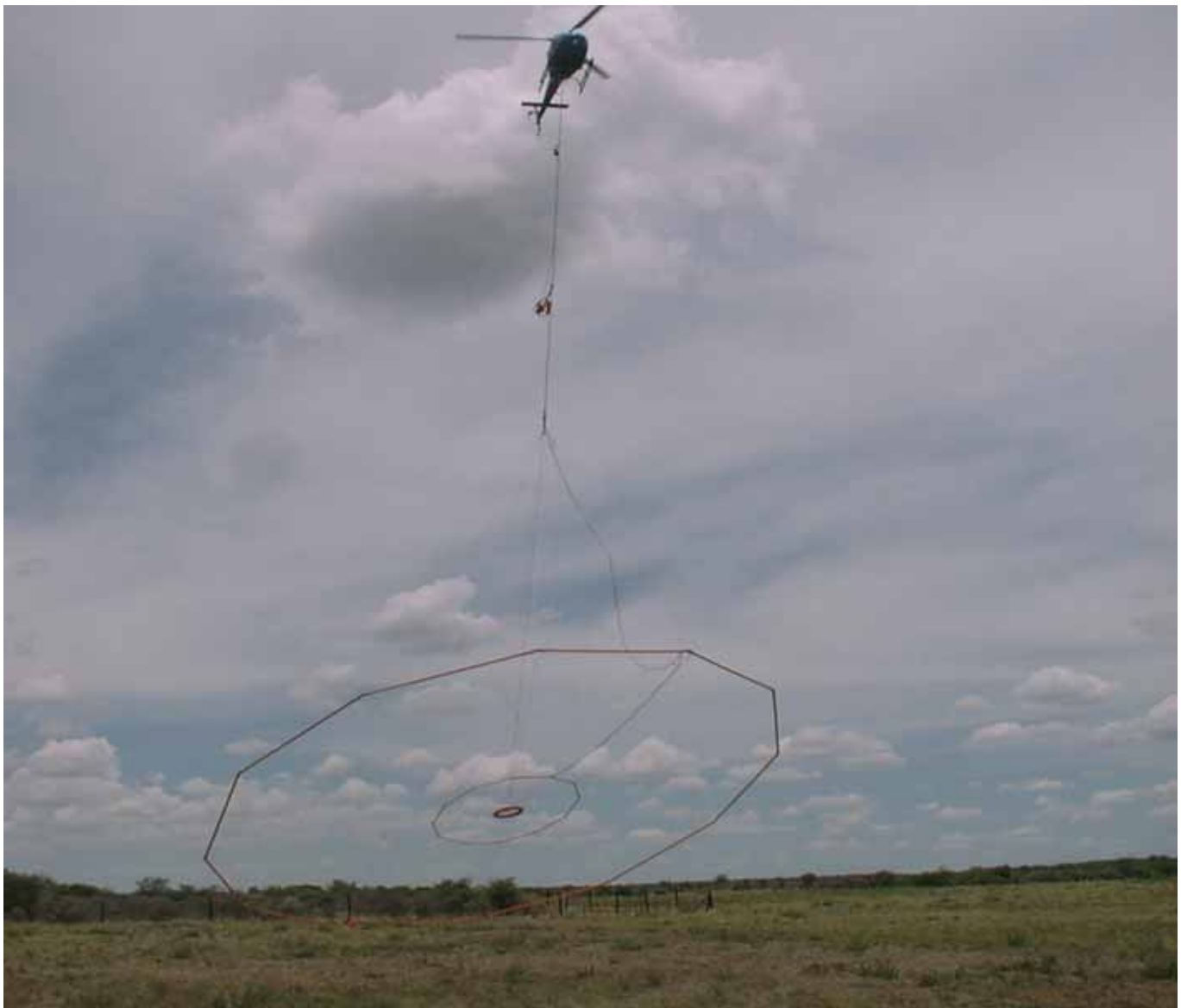
An airborne electromagnetic survey under way at the Segwagwa project, Botswana
