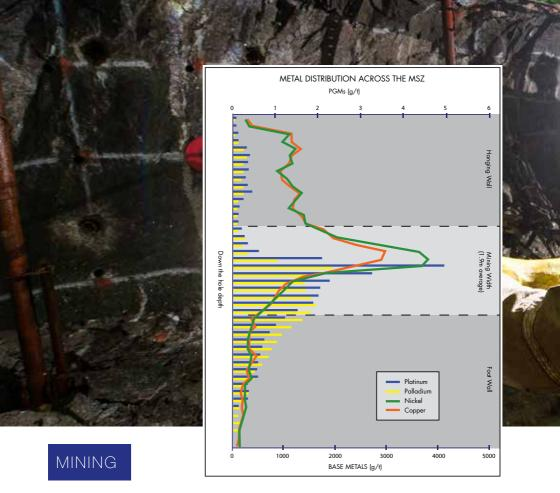
Mimosa holds contiguous mining rights over 6 591 hectares on the North Hill, the South Hill, Mtshingwe Block and Far South Hill orebody areas. The orebody is shallow and mining commences at a depth of 150 metres below the surface and extends to a depth of approximately 200 metres. The bord and pillar mining method is employed and stoping widths average around 2 metres. Mining bords advance along the strike.
