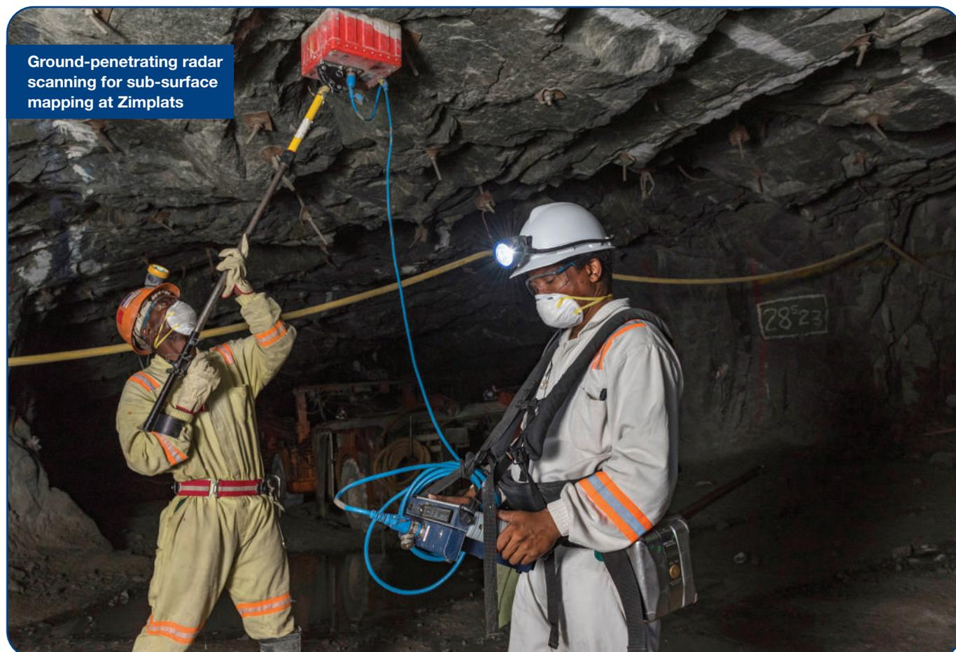
Ground-penetrating radar scanning for sub-surface mapping at Zimplats
