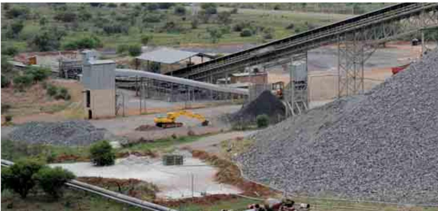
The stockpile offers surge capacity between the mining and plant process
