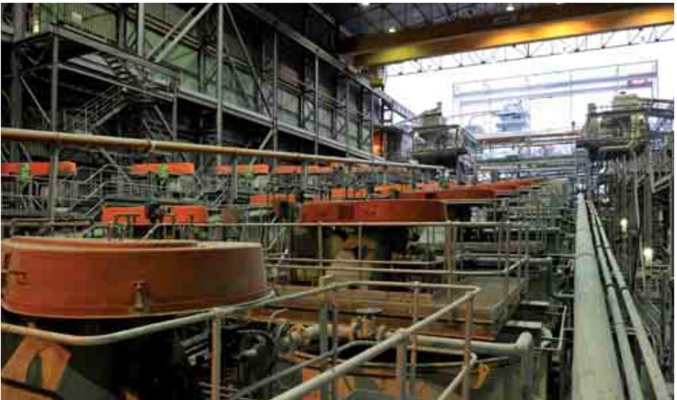
Flotation cells at BRPM's concentrator
