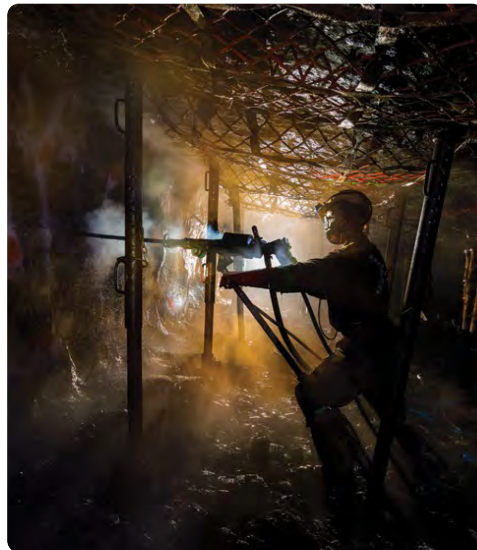
Stope drilling at BRPM North shaft, UG2 reef
